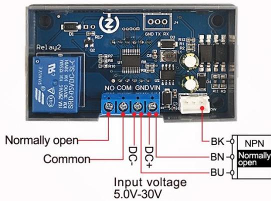
6.Trigger of serial port signal—mode of connection:
