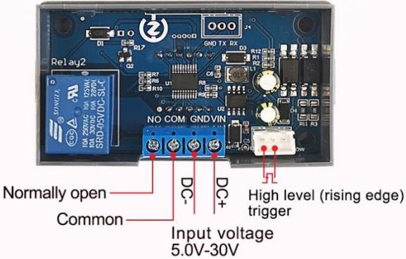
4.PNP sensor signal trigger—mode of connection:
