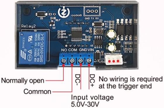
2.Passive switch signal trigger— mode of connection:
